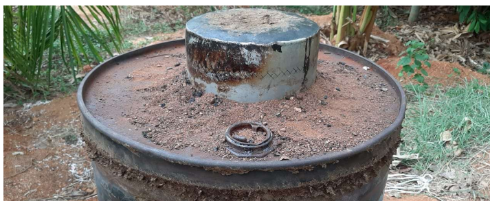
The cooling phase of the drum Biochar furnace in an IBBN field school
